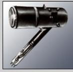
One of the first models of the super-conoscopethe transmitting television tube, made in P.Shmakov's laboratory. 1937
